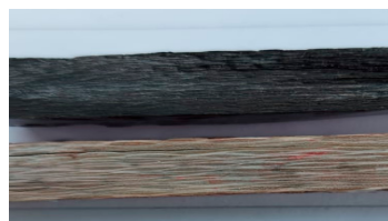
Figure 4. Rectangular glass and carbon composite samples.
