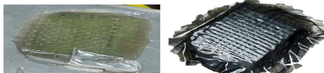
Figure 3. Glass and carbon composites after curing.
