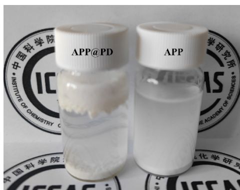
Figure S2. Dispersion of APP and APP@PD in water after resting for 1h.
