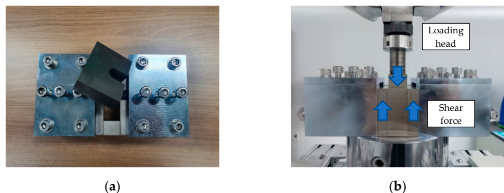
Figure 6. Shear strength test of CFRP rebar based on ASTM D7617. (a) shear jig; (b) test set-up.
