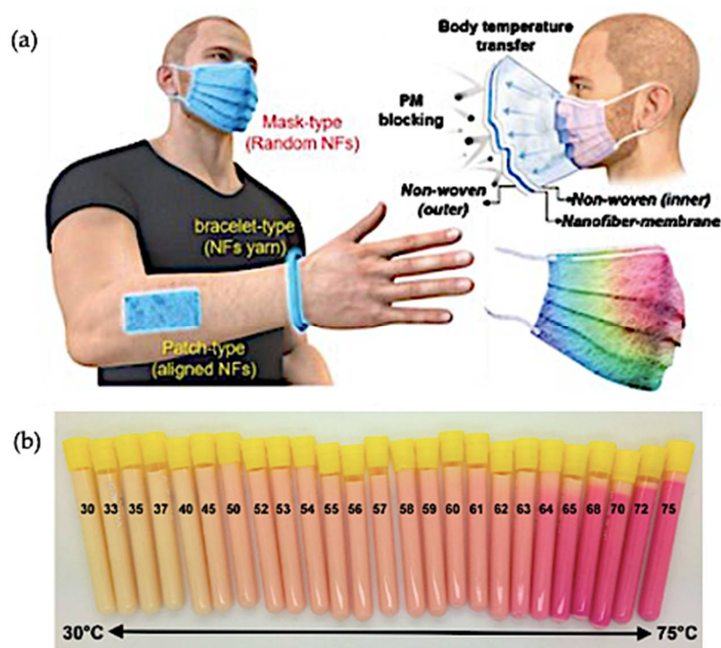
Figure 13. Innovative thermochromic material in health and medical device applications. (a) Fabrication process of reversible thermochromic nanofibrous membrane—potential applications in respiratory masks, patches, and bracelets [85,90]. (b) Development of tissue-mimicking thermochromic phantoms for MRI-imageable and HIFU-compatible temperature sensing [219–221].
