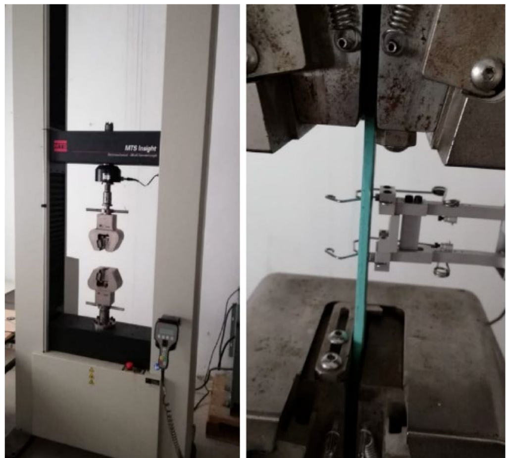
Figure 6. MTS insight tensile test machine with the specimen between the grips.
