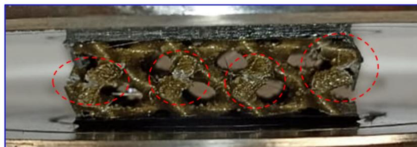
**Figure 10.** Compression sample of 20% relative density gyroid core sandwich during test.
