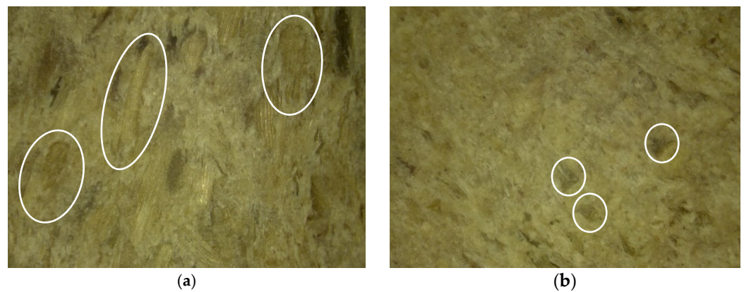
Figure 11. Microstructure of the surface of the polymer composite filled with wood flour. (a)—Control, (b)—Control + Modifier.
