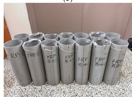
Figure 7. Failure modes of tensile test specimens: (a) detail of specimen; (b) failure mode within upper jig; (c) failure mode of FRP-25-4-1; (d) failure mode of tensile test all specimens.
