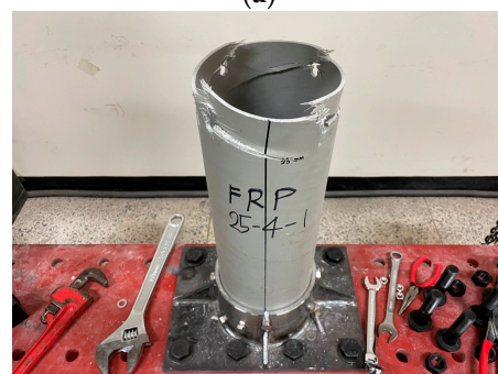
Figure 7. Failure modes of tensile test specimens: (a) detail of specimen; (b) failure mode within upper jig; (c) failure mode of FRP-25-4-1; (d) failure mode of tensile test all specimens.
