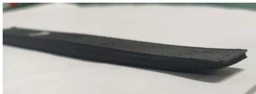
Figure 11. Printed samples (warpage deformation).
