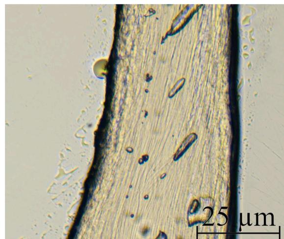
**Figure 3.** Morphology of a just spun non-precipitated extrudate formed from an 18% blend solution in NMMO (70% PAN/30% cellulose,  $T = 120\text{ }^{\circ}\text{C}$ ).
