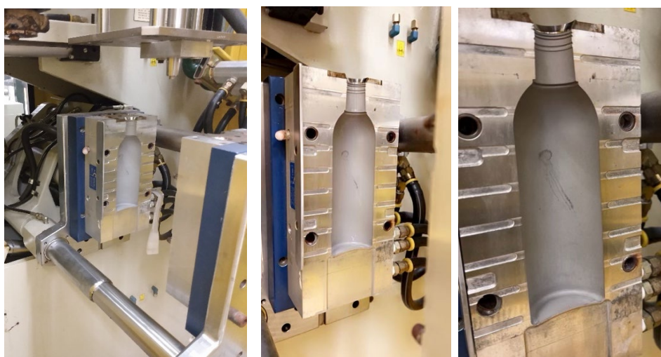
Figure S3. Bottle mold design.
