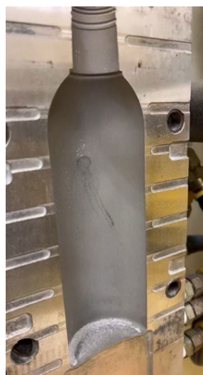
Figure S5. The bottle mold after the application/deposition of the \text{Mg}(\text{OH})_2 dry powder.
