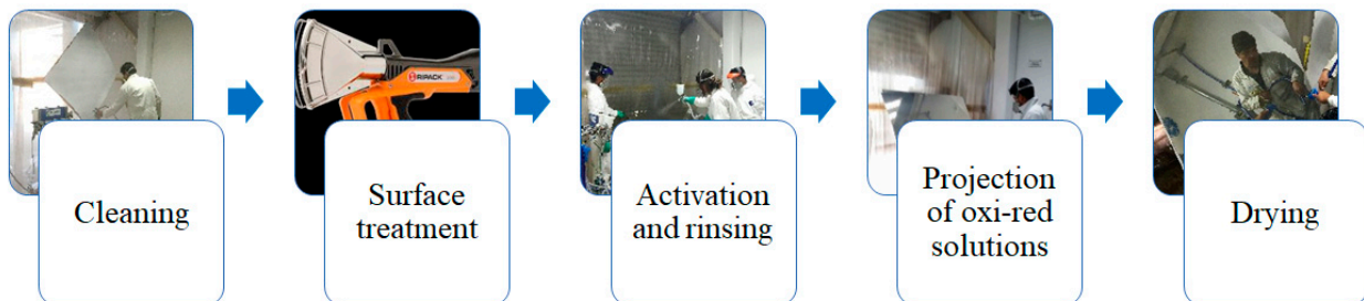
Figure 2. Diagram of the DCP metallization process.
