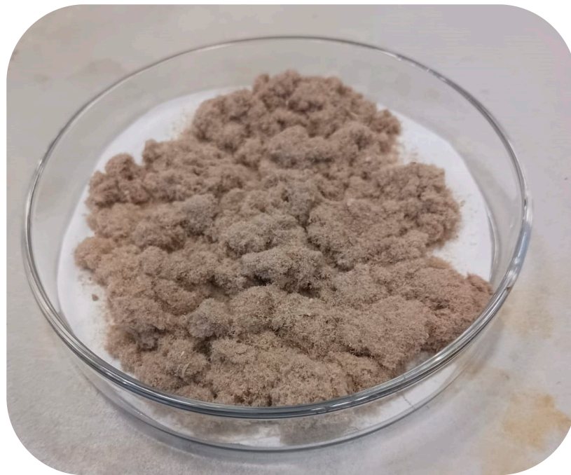
Figure 2. The appearance of a WP sample after the grinding process.
