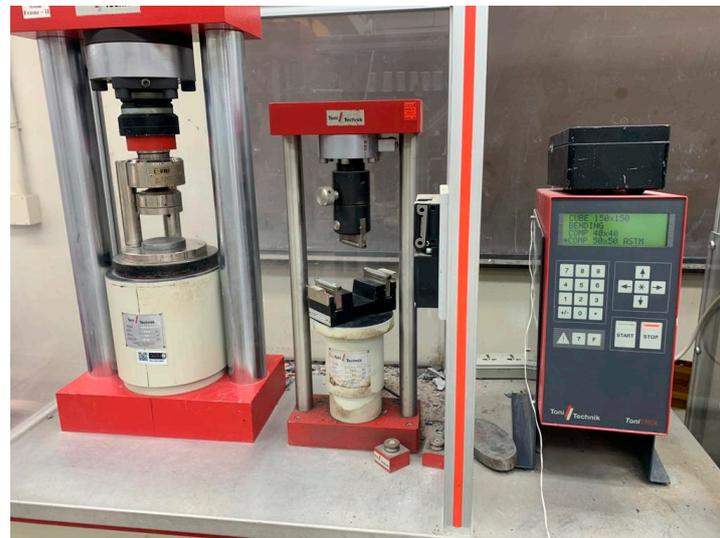
**Figure 4.** Universal testing machine.
