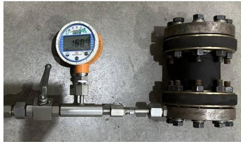
**Figure 4.** Balanced performance test of the FRR pipe.
