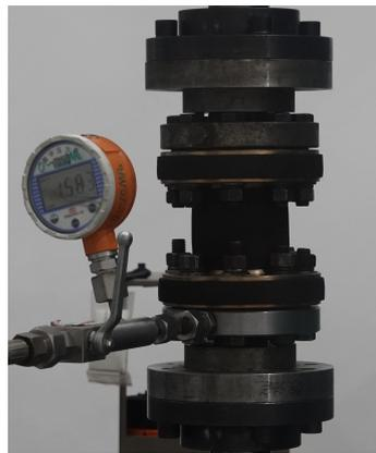
**Figure 8.** Expansion phenomenon of the FRR pipe under compression load and internal pressure.
