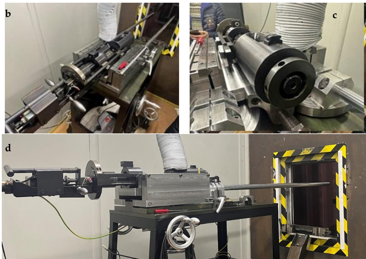
Figure 4. Test range configuration (a); test stand with a test barrel (b–d).
