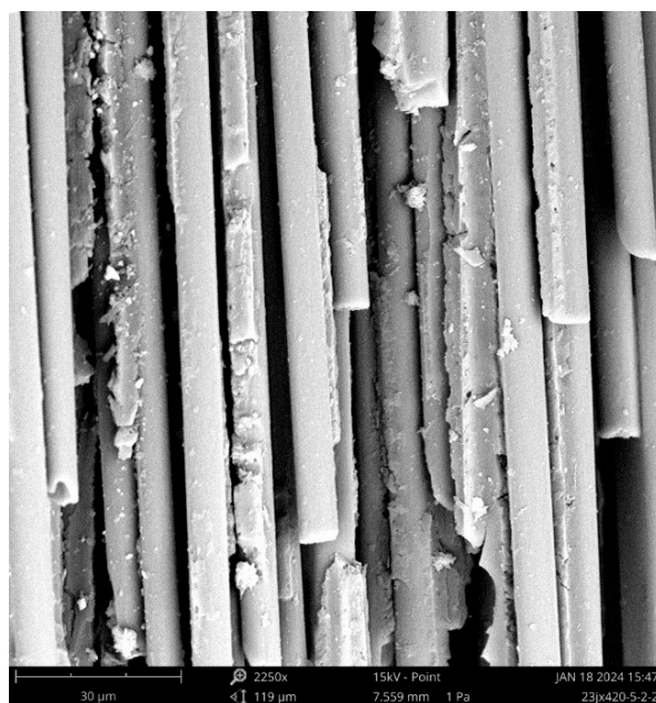
Figure 5. Morphology of CFRP rod after fracture.
