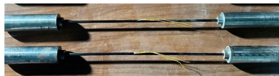
Figure 1. Tensile test specimen of CFRP rod.
