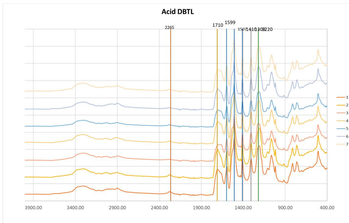
Figure S1: FTIR spectra of foams using acid liquefied polyol and DBTDL as catalyzer;
