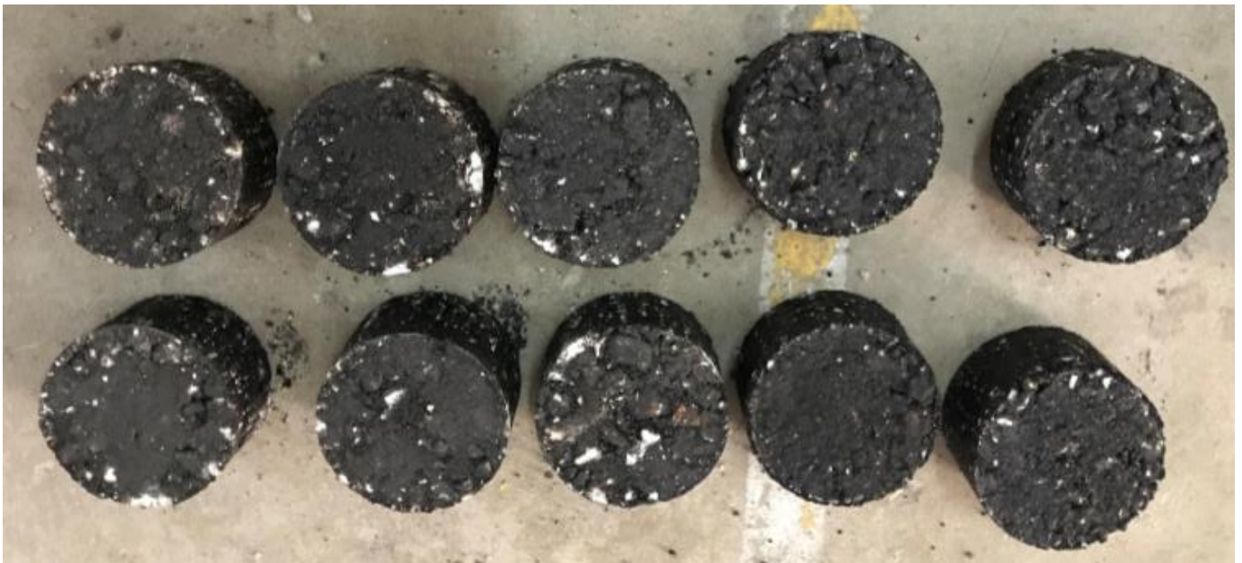
Figure 3. Compacted samples of Marshall stability.
