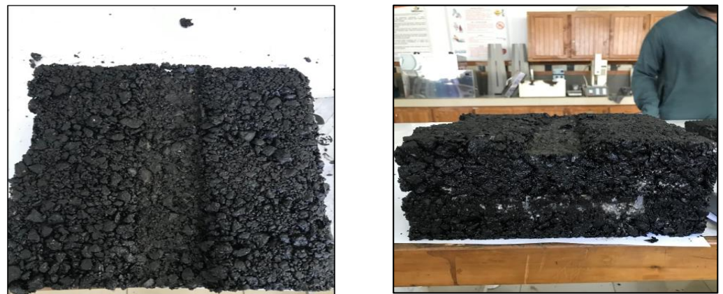
Figure 9. Slab specimens in wheel-tracking tests.
