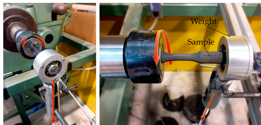
Figure 5. Rotational bending fatigue equipment. Sample undergoing the test.
