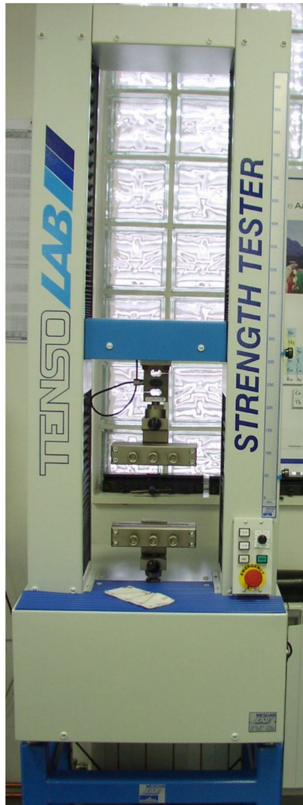
Figure 14. MesdanLab Strength Tester, S.p.A., Italy, Tensolab 3000, used for HRN EN ISO 2062:2010 Textiles—Yarns from packages—Determination of single-end breaking force and elongation at break using constant rate of extension (CRE) tester (ISO 2062:2009; EN ISO 2062:2009) [55,56].
