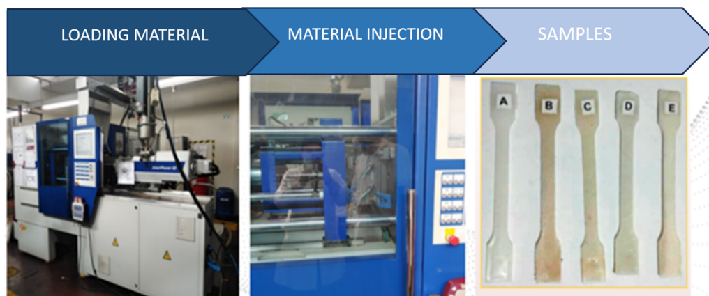
Figure 2. Injection molding process of test specimens. (A) LDPE 100%, PS 0.0%, MFCA 0.0%; (B) LDPE 84.95%, PS 15%, MFCA 0.05%; (C) LDPE 84.85%, PS 15%, MFCA 0.15%; (D) LDPE 84.7%, PS 15%, MFCA 0.30%; (E) LDPE 85%, PS 15%, MFCA 0.00%.
