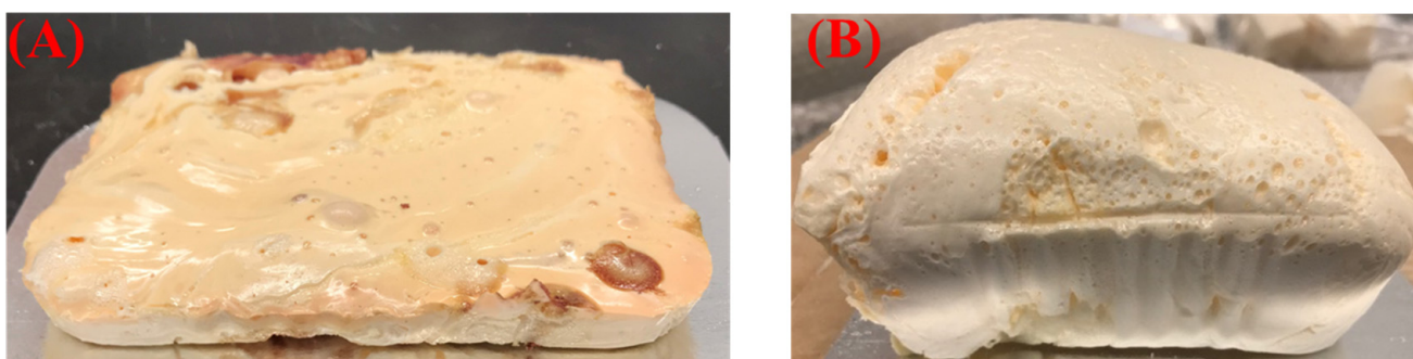
Figure 3. Phenolic foams formulated with (A) HFO-1336mzz (E) (PF OP1) and (B) HFO-1336mzz (Z) (PF OP2) blowing agents.
