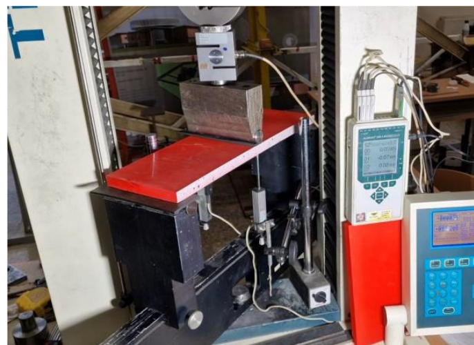
Figure 8. The three-point bending test setup.
