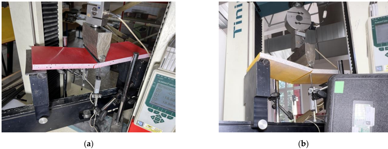
Figure 14. The failure patterns of the single-part specimens: (a) PLA (S-1); (b) LW-PLA (S-3LW).
