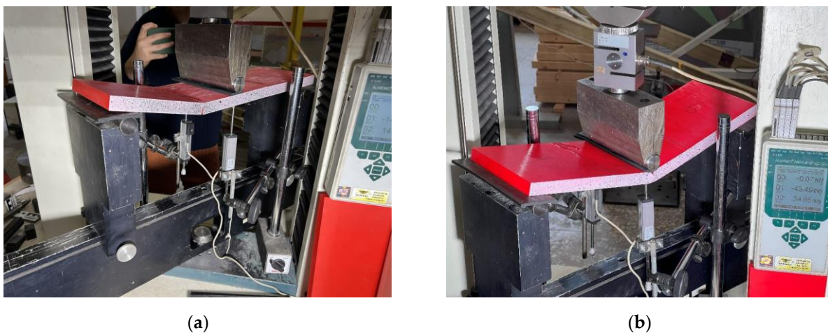
Figure 15. The failure patterns of the three-part bending specimens with different arrangements of the printing pathways regarding the adhesive joints: (a) Perpendicular (F1-2); (b) Parallel (F2-1).
