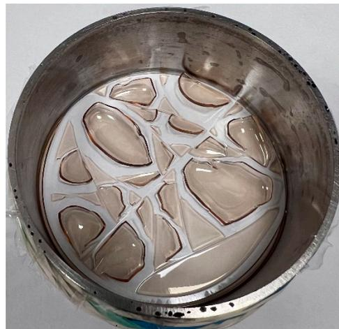
**Figure 5.** Photograph of a solution-cast polymer film based on poly(NBpin-co-NBI) (40:60 mol.%).
