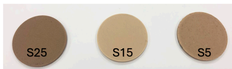
Figure 2. Specimens manufactured for the water absorption tests: 25 wt.% wood (S25), 15 wt.% wood (S15), 5 wt.% wood (S5).
