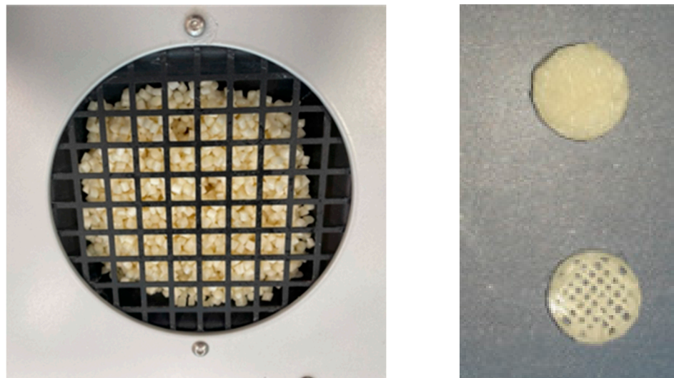
Figure 2. (Left)—mixture of PLA/PHB and OLA in pellets, (Right)—printed samples solid/porous.
