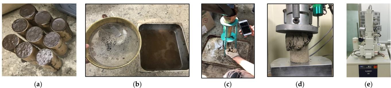
**Figure 2.** Sample preparation and testing procedures: (a) sample preparation, (b) mixing stability test, (c) flowability test, (d) unconfined compressive strength (UCS) test, (e) SEM examination.
