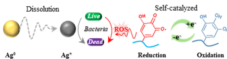
Figure S4. Proposed synergistic antibacterial properties based on sustainable dissolution of AgNPs and release of reactive oxygen species (ROS) generated from the redox reactions of catechol groups in polyphenols.
