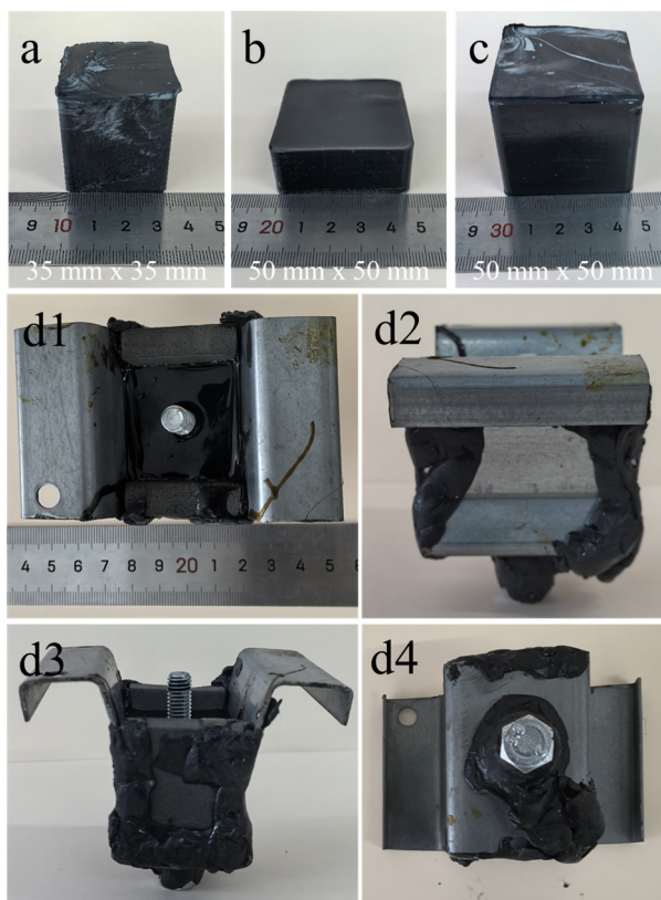
Figure S4. Different structural adhesive applications: rectangular structural adhesive measuring: (a) 35 mm x 35 mm; (b) 50 mm x 50 mm; (c) 50 mm x 50 mm at different heights. (d1~d4) Digital photograph of the self-made metal frame with structural adhesive.
