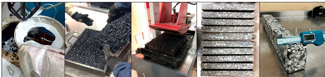
Figure 5. Preparation of prismatic test specimens.
