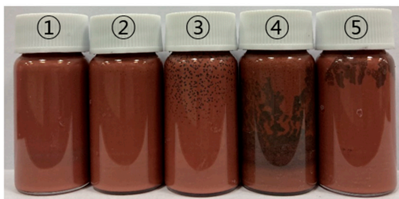
Figure 8. Phase separation of Cu sintering paste containing 450 mg/mL (acidic acid/solvent) with different epoxy/acidic additive ratios: ① 0:10, ② 2:8, ③ 4:6, ④ 6:4, and ⑤ 8:2.
