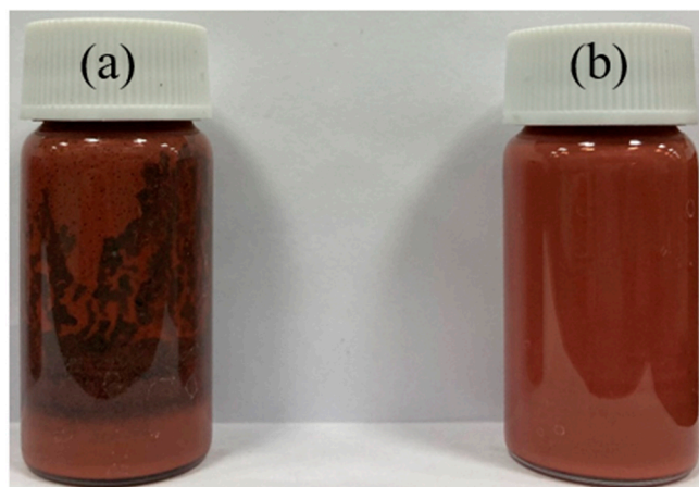
Figure 9. Phase separation of Cu sintering paste seven days after fabrication depending on storage conditions: (a) room temperature and (b) 4 °C.
