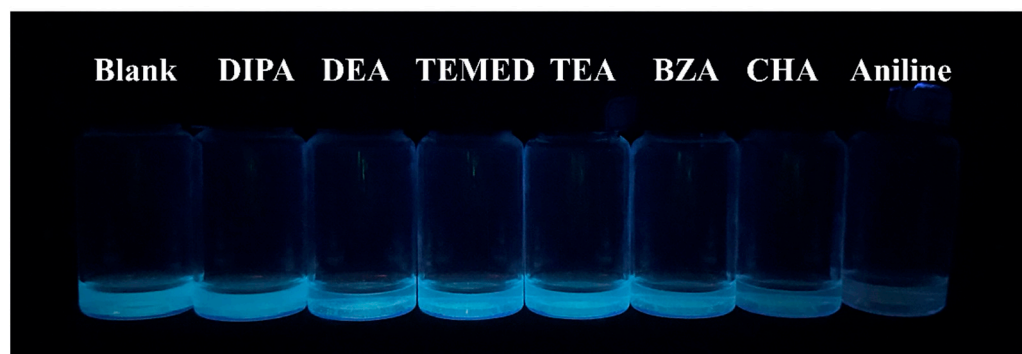
Figure 8. Fluorescence of PPCM solution under UV lamp (365 nm) after addition of different amine compounds.
