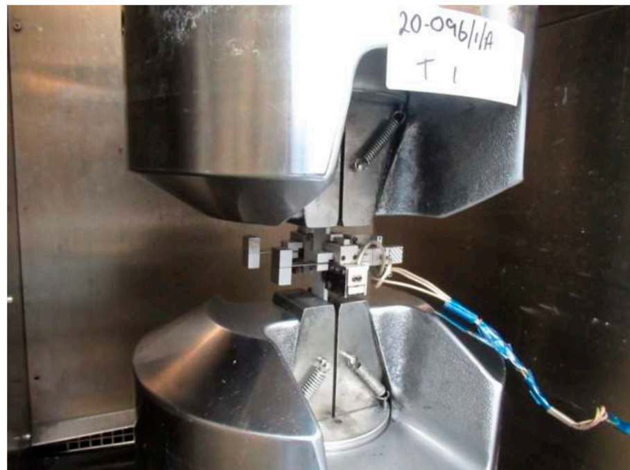
Figure 2. Test setup for the static test on polymer composite samples in the longitudinal direction.
