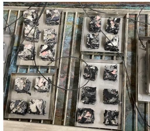
**Figure 8.** (a) One cycle of freeze–thawing of samples. (b) Samples laid out in freezing chamber.
