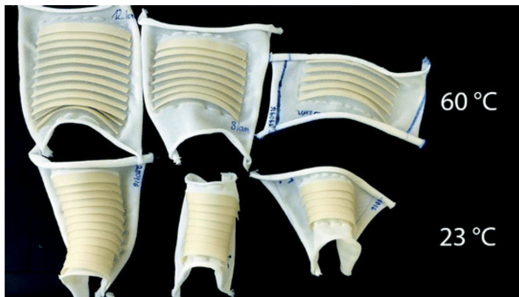
Figure 7. 4D textile with and without stimulus: heat [59]. Reproduced from [59], with permission from Springer Nature and Copyright Clearance Center, 2023.
