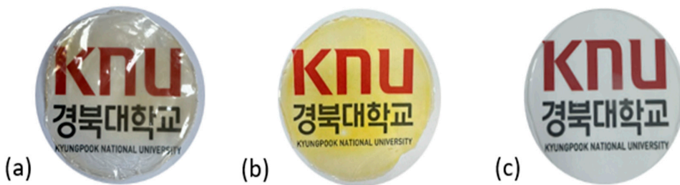
Figure 2. The appearance of (a) optimized bilayer pectin/PLA film, (b) single pectin film, and (c) single PLA film.
