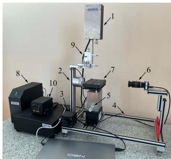
Figure 5. ACAM automatic contact angle measurement system: 1—dispenser module; 2—light source; 3—lighting intensity regulator; 4—base; 5—table raising regulator; 6—camera; 7—table with a substrate; 8—chief controller; 9—horizontal and vertical needle adjustment systems; 10—engine of the dispenser module.
