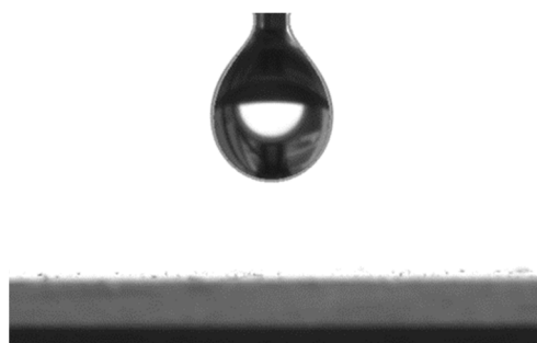
Figure 6. Image of a bitumen drop dosed to determine surface tension.
