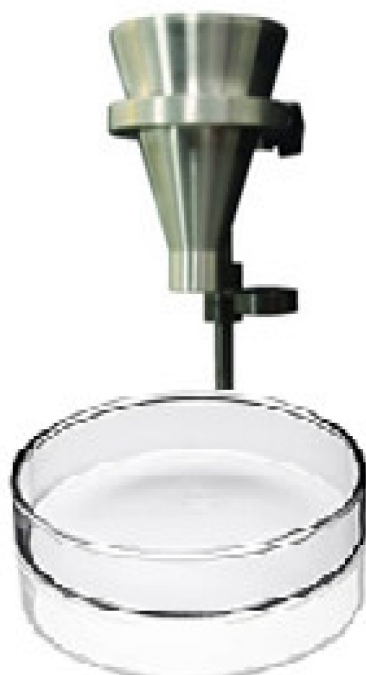
Figure 4. Bulk density measuring apparatus.
