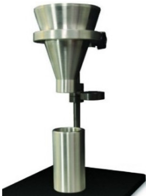
Figure 3. Mass flow rate measuring apparatus.
