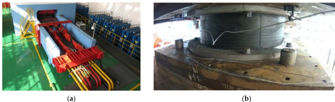
Figure 3. Compression-shear test of specimen: (a) Multifunctional apparatus; (b) Installation of the specimen.
