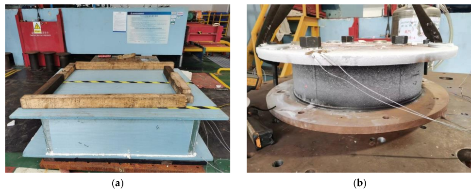
Figure 2. Cooling process of specimen: (a) Thermal insulation device; (b) Cooling specimen.
