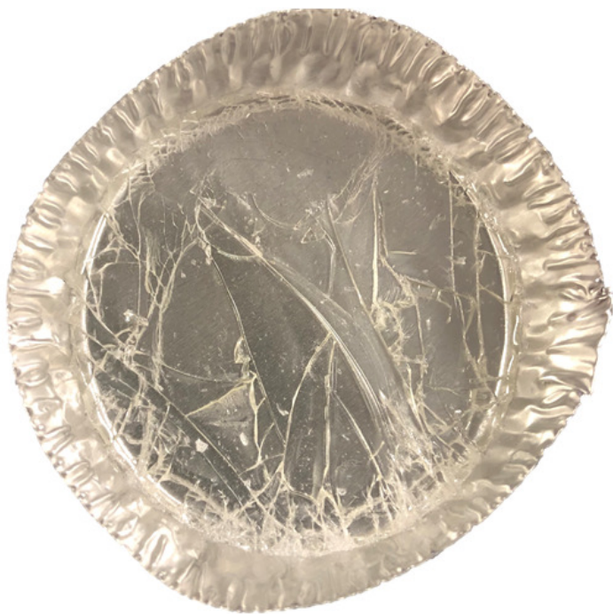
Figure S 4 Sample of LDO/PAG mixture in an aluminum dish, polymerized at ambient temperature (PAG = 0.1 wt%, 1 minute irradiation, 60% relative humidity).
