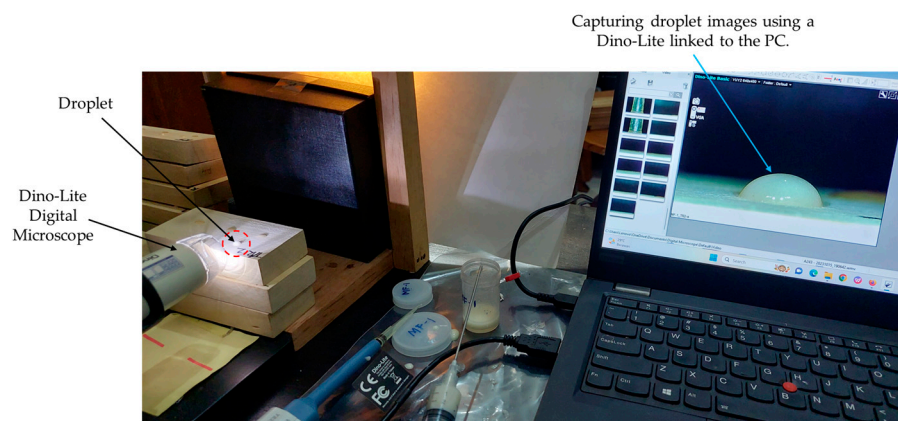
Figure 2. Capturing droplet distribution and change patterns with a Dino-Lite Digital Microscope (Am 2111 series) adjusted for 40× magnification.
