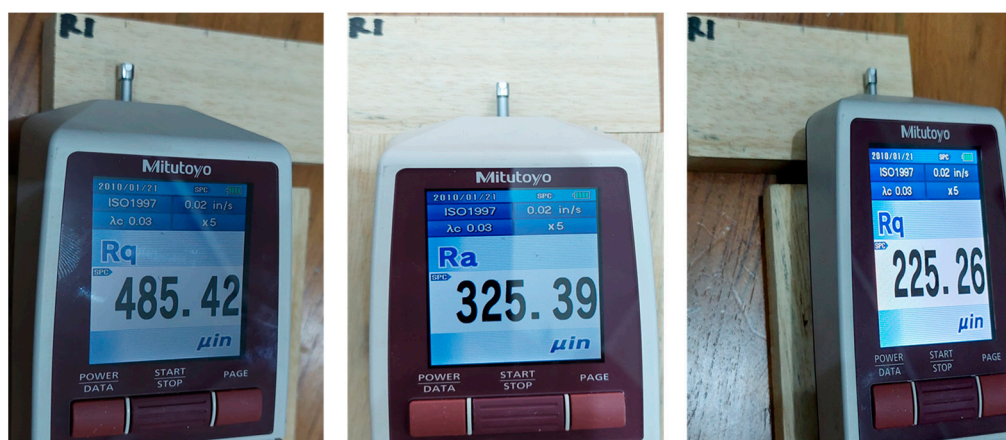
Figure 1. The surface roughness measurement of Jabon wood specimens in three different positions using a portable stylus-type profilometer (Mitutoyo SurfTest ® SJ-210).
