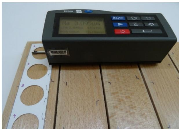
**Figure 5.** Measuring the roughness of the wood-coated surface.
