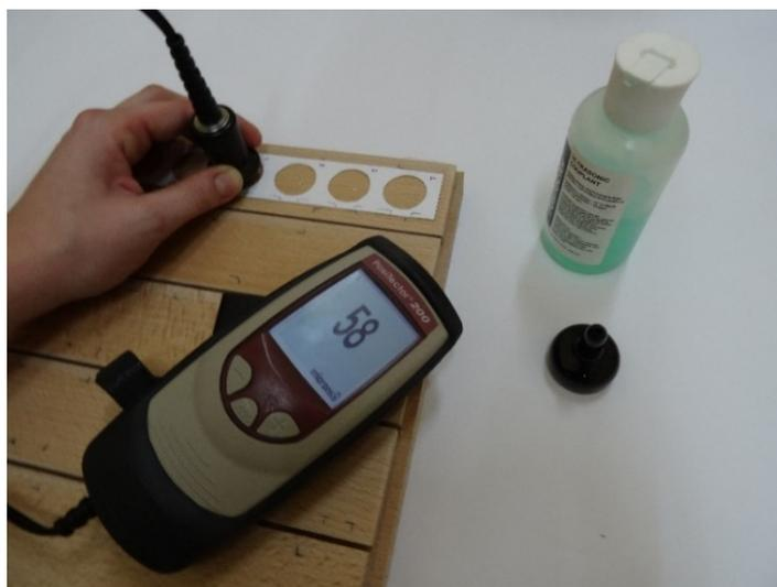
**Figure 2.** Dry film thickness measurement of water-based transparent acrylic coating.
