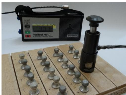
**Figure 4.** Determination of WTAC adhesion strength by the pull-off test.
