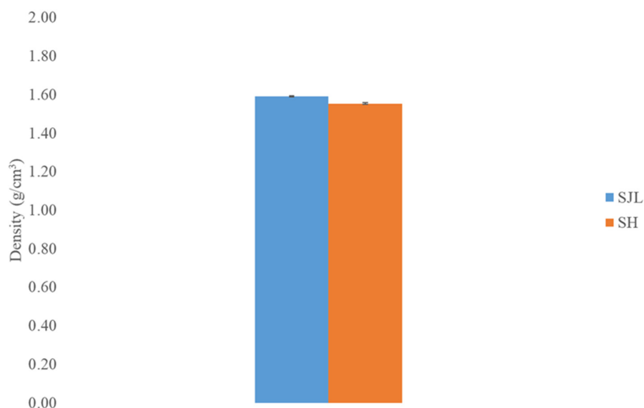
Figure 3. Density of Spartium junceum L. (SJL) and Sida hermaphrodita (SH) fibers. Error bars represent 95% confidence interval.
