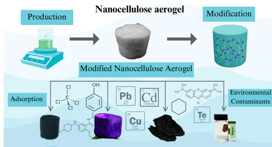
Figure 8. Production and application of modified nanocellulose aerogels in the adsorption of environmental contaminants. Adapted from [38,39,49,63,70].
