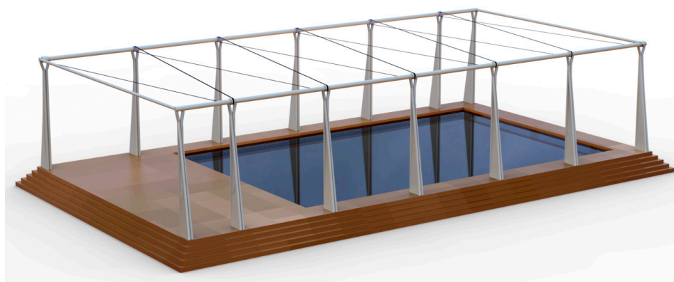
Figure 31. Swimming pool cable roof with CFRP Continuous Band Winding System.
