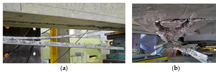
Figure 7. Longitudinal fracture of the CFRP profile web in beams: (a) B60-214-1T-30; (b) B60-214-2T-30.
