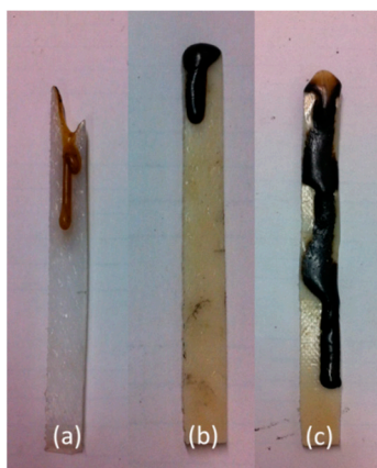
Figure 4. PA6 sample tested at an Oxygen Index (OI) below 28 vol% (a); the PA6/GAS 2.5%/MPP 2.5% sample tested at OI between 23 and 30 vol% (b) and between 31 and 36 vol% (c).
