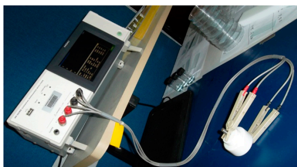
Figure S2. The complete EIS measurement setup using a HIOKI IM3590 instrument.
