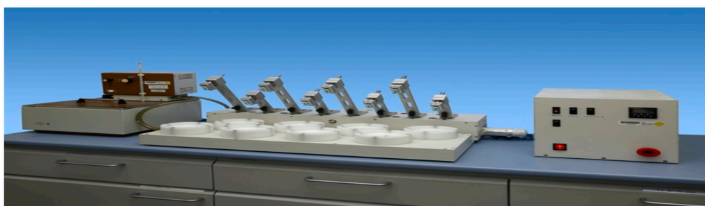
Figure 4. Willytec tooth-brushing simulator for abrasion tests.
